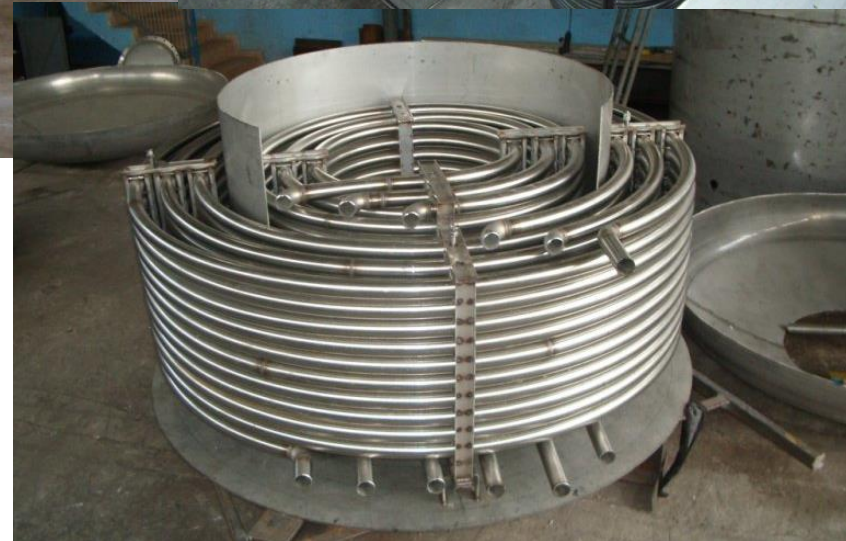
Olive Oil Heat Exchanger
