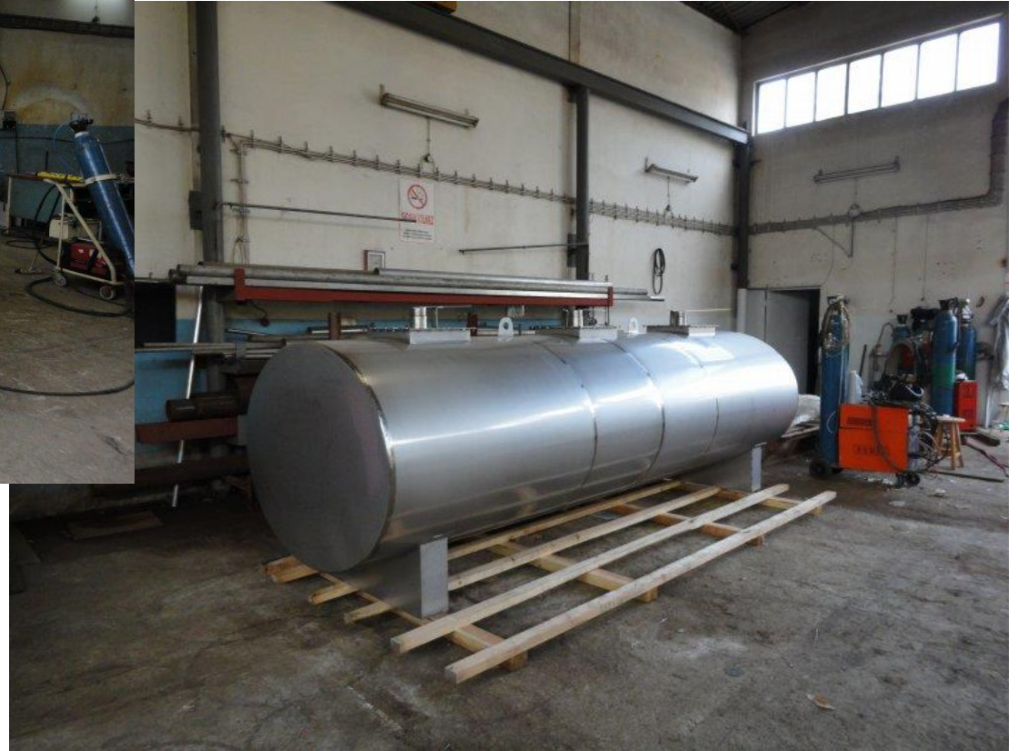
Olive Oil Tank
